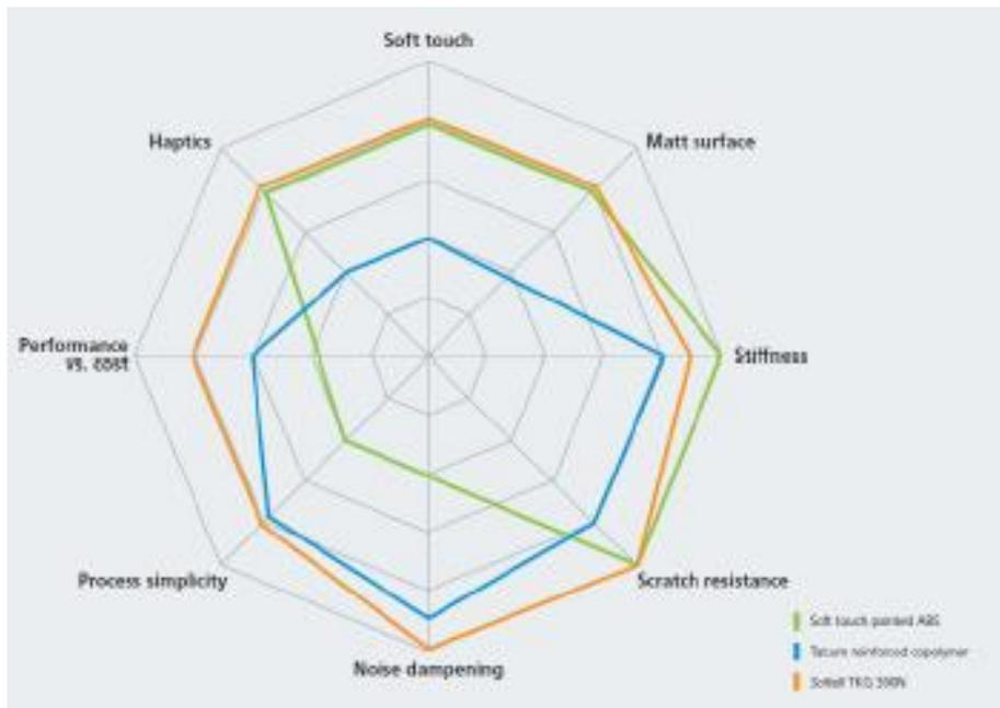
Waterborne soft-touch coatings are typically achieved by combining flexible polyurethane dispersions of high molecular weight with flexible hydroxyl-functional pre-polymers and crosslinking them with flexible, water-dispersible poly-isocyanates. The two component urethane technology enables customers to get the optimum combination of properties without compromise by providing a coating that feels soft but has excellent durability.
