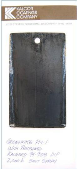
**4c. Waterborne Coating with Phosphate vs. Thermal Diffusion: 720 hours ASTM B117 Salt Spray**
