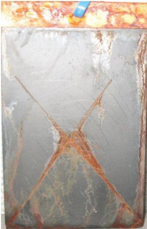
**Figure 5b. PM-1 Thermal Diffusion with adhesive top coat following 1,000 hours salt spray**
