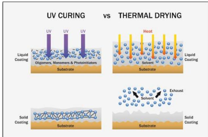
In addition, UV coatings contain photo-reactive agents called photoinitiators. When these photoinitiators are exposed to high intensity “light” in the Ultraviolet region of the spectrum (usually around 250-400 nanometers) the energetic UV rays cause some atomic bonds on the photoinitiator molecules to break - quickly.
